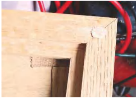
STEP 20. You can now glue and screw the corners. You need to add glue and a 'foot' on the corner. The foot can then be sanded off and cut
